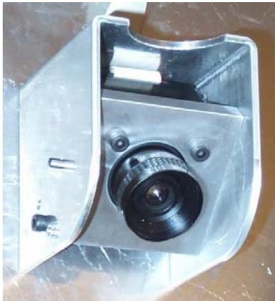
Figure 5.41 The camera installed in the special designed mounting base.
