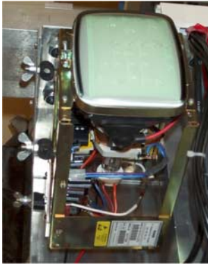
Figure 3.86 The monitor is fitted to the back plate with 3 rubber vibration dampers.
