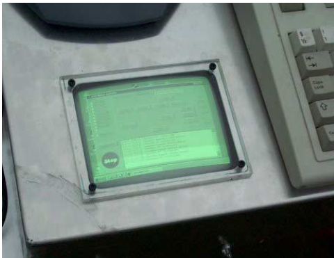
Figure 4.16 The 5" monochrome VGA monitor protected by plexiglas
