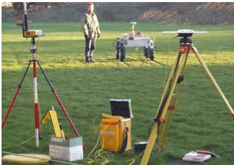
Figure 5.14 RTK base station. GPS antenna to the right, computer in the middle and radio transmitter to the left.
