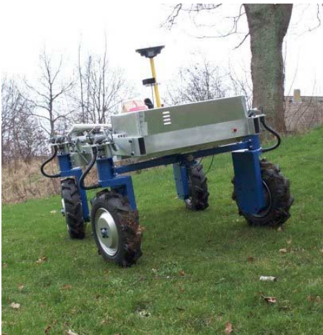
Figure 8.5 Flexible steering and off road capabilities with 4WD and 4WS.
