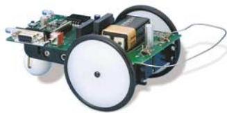
Figure 2.7 Robot with 2WD differential steering.
