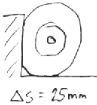
Figure 3.12 Deformation of the tyre, when hitting an obstacle with 1 m/s.
