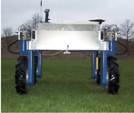
Figure 8.1 Designed for in-row driving with slim wheel modules and good ground clearance.
