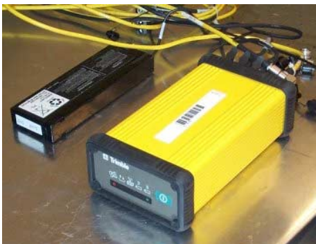
Figure 5.16 The Trimble RTK rover on the vehicle.
