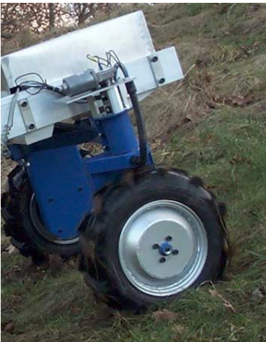
Figure 5.9 Wheel spin will not be discovered when calculating travelled distance.
