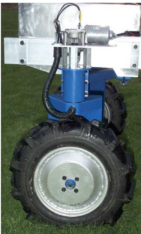
Figure 8.2 A DC motor is used to steer each wheel.
