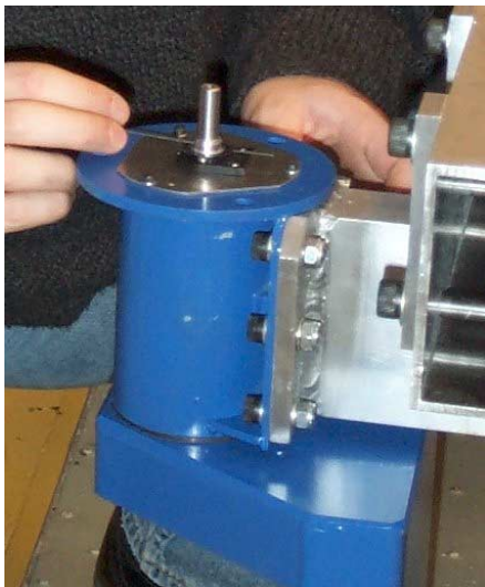
Figure 5.7 Adjusting index position on a steering motor encoder.
