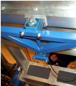
Figure 3.71 Bolting the Rosta bearings to the front module.
