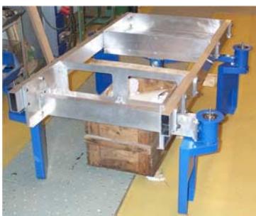
Figure 3.88 The chassis with the partly assembled wheel modules.
