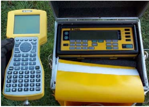
Figure 5.15 The Trimble RTK base station computer and controller.
