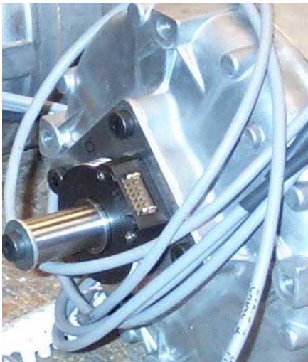
Figure 5.8 Encoder mounted on the Honda motor
