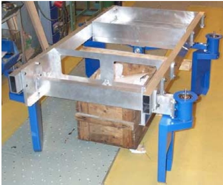
Figure 3.95 Chassis and wheel modules assembled by the workshop technicians.
