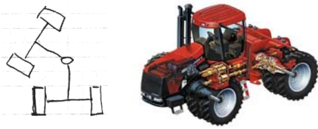
Figure 2.9 Tractor with articulated steering and the steering principle.
