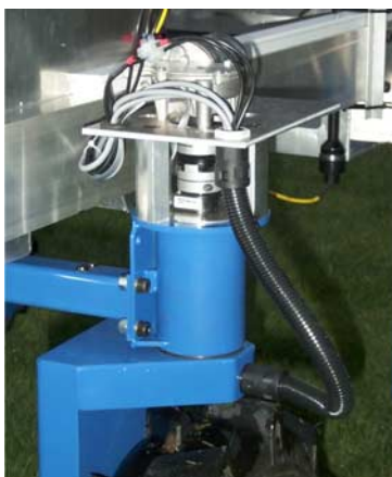
Figure 3.50 The wires are going through a conduit to the motor bracket.
