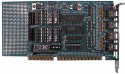
Figure 5.6 The quadrature decoder interface card.
